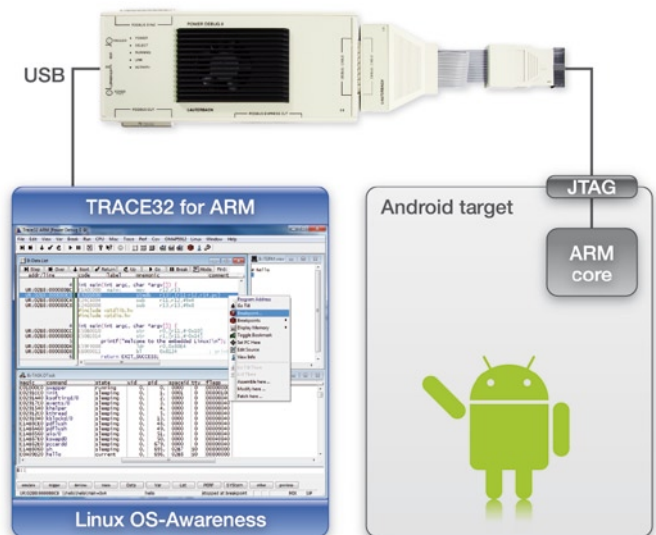
Fig. 6: In stop-mode debugging, the debugger communicates directly with the processor on the Android hardware platform.
