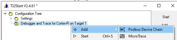
4. Add the **POWER DEBUG PRO** to the **Podbus Device Chain**.
