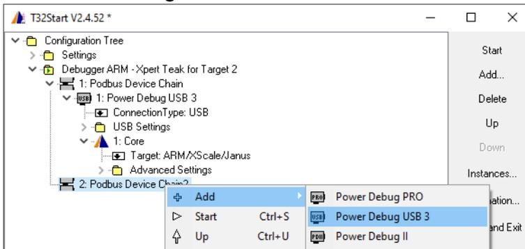
9. Assign the second **Core** to the second **Power Debug USB3**.
