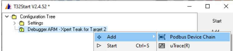
4. Add a **Power Debug USB3** to the **Podbus Device Chain**.
