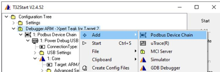
8. Add a **Power Debug USB3** to the second **Podbus Device Chain**.
