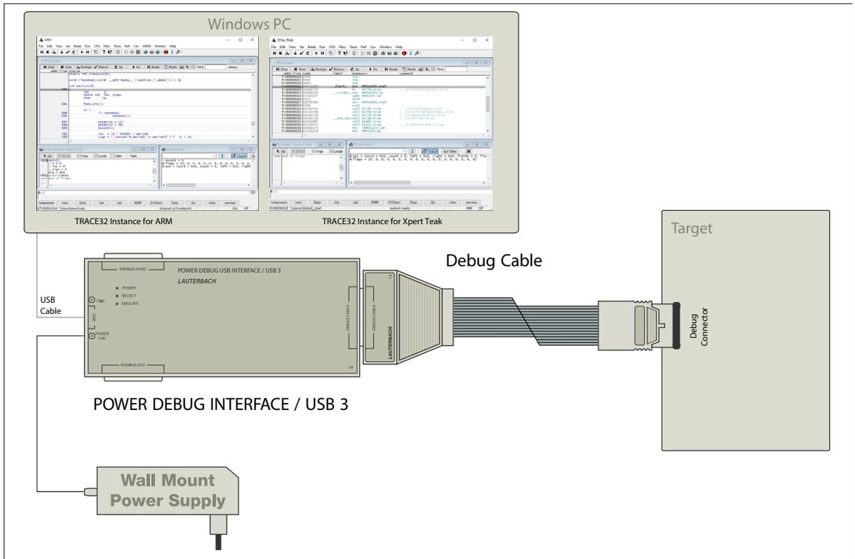
If you want to debug two identical cores, you can also do this with two TRACE32 instances (homogeneous AMP).
