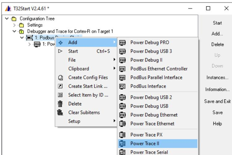
6. Assign a Core to the **Power Debug PRO**. The reason for this assignment is that the TRACE32 driver software/JTAG handler runs on the Power Debug PRO module.
