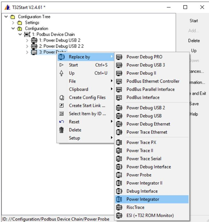
Please note that LAUTERBACH devices which have a **PODBUS SYNC** connector (instead of **PODBUS IN**), require an own power supply and connection to the host (USB or Ethernet). These devices cannot be added to a single **Podbus Device Chain**. Each device has to be configured as a separate **Podbus Device Chain**. The type of the PODBUS connection is printed on the device.
