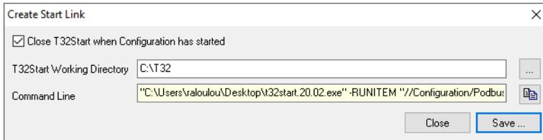
After the link is executed, T32Start will appear and start the connected item and all sub-items. After starting, T32Start will be closed automatically based on the settings.
