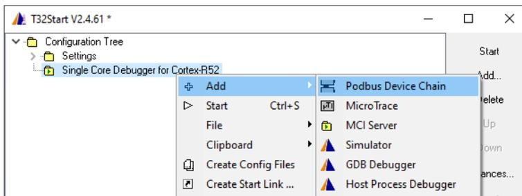
4. Add the Power Debug USB3 to the **Podbus Device Chain**.
