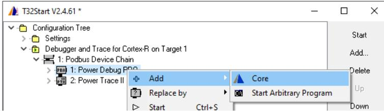
Because two devices are used for debugging, both of them have to be included in the **Podbus Device Chain**.
