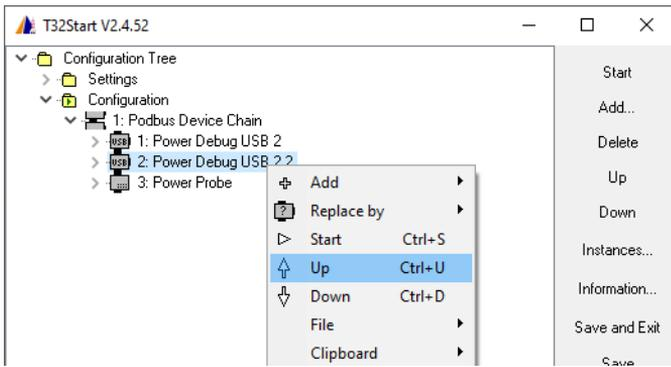
Every device has a menu item **Replace by** to exchange it by a another device. While the exchange takes place the settings of the device are kept if possible.
