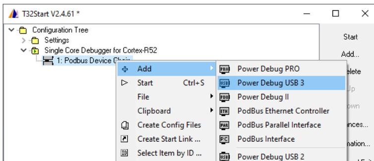
5. Assign a Core to the **Power Debug USB 3**.
