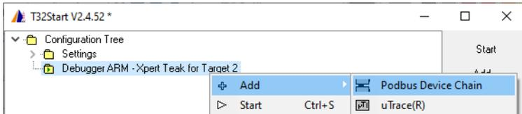
4. Add the Power Debug USB3 to the **Podbus Device Chain**.
