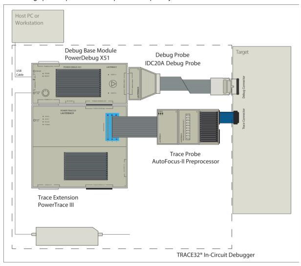
Details on the required connector type and pin assignment on the target system can be found on the Lauterbach website <a href="https://www.lauterbach.com">https://www.lauterbach.com</a> in the description of the corresponding debug or trace probe. The available adapters/converters that convert to a different connector type or pinout are also listed there, if this is required for the target system.
