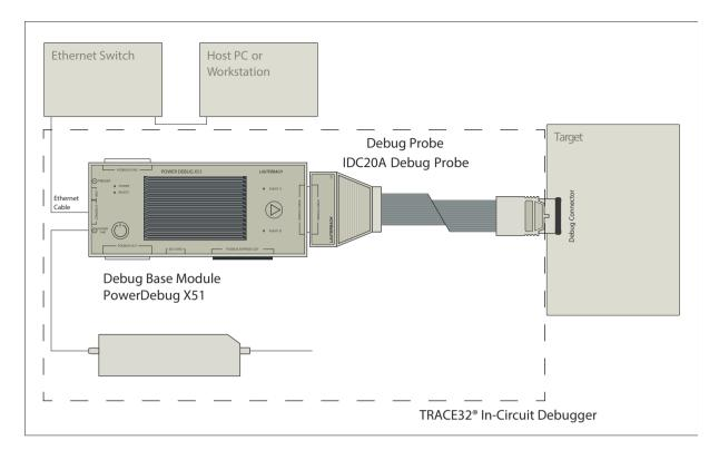
To obtain additional off-chip trace functionality, the "PowerDebug X51" debug base module can be supplemented by connecting a **trace extension** to the "PODBUS EXPRESS" connector and a trace probe. These extensions can be classified technologically as parallel or serial.
