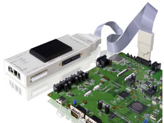
Figure 4: JTAG debugger with the target system: This is how a hardware debugger is connected to the target system.
